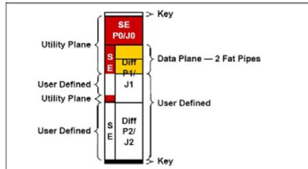
Figure 14.3.1-1 Peripheral Slot Profile SLT3-PER-2F-14.3.1
