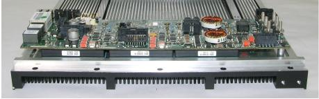
View of power supply mounted to heat exchange bulkhead. Chassis has option for 1 or 2 power supply modules or 1 power supply module and 1 hold up module.
