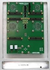
Ribbon cable I/O connectors on rear side of front panel
