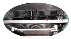
Above: View of machined card guides, heat exchange bulkhead, and rear exhaust fans
