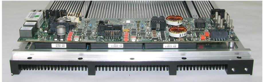
Above: View of machined card guides, heat exchange bulkhead, and rear exhaust fans
